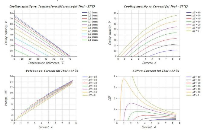
To cool the inside of the reactor, a positive voltage must be applied to the red cable opposite the black earth cable. To heat the inside, a negative voltage can also be applied.
