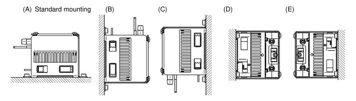
Installation top side down is prohibited and may cause damages to the device.
