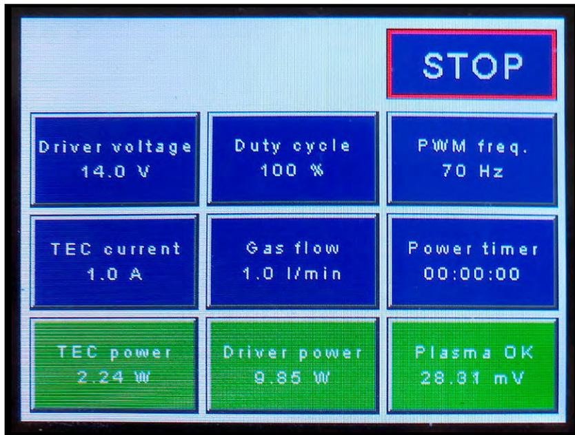
After selecting the “RUN” menu item in the start menu, the screen changes to the process menu with the “STOP” field circled in red. A screenshot is shown on the left side.
