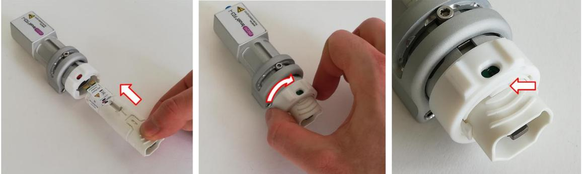
Grip the module carrier as shown and place it on the driver housing by sliding it onto the two locating pins from the front and then pressing it firmly against the driver housing.
