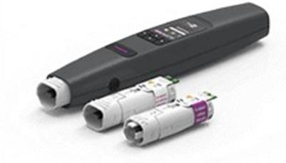
The PZ3 PiezoBrush is a compact hand-held plasma device that was developed for use in laboratories, advance development and assembly in short production runs. With a maximum power consumption of 18 W, Piezoelectric Direct Discharge (PDD®) technology is used to generate cold-active plasma at a temperature of less than 50 °C.
