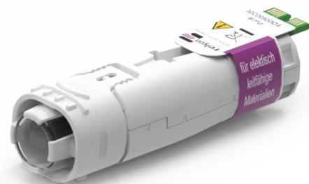
The device can only generate a surface activation if an electrically conductive substrate is in front of the device within the range of the permissible working distance. This is approx. 0.5 to 2.0 mm. If the distance is greater, plasma generation may not be possible under certain circumstances, depending on the material and geometry of your substrate.
