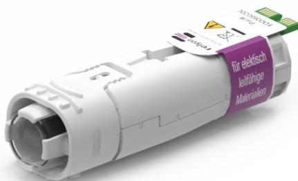
The device can only generate surface activation if there is an electrically conductive substrate in front of the device within the range of the permissible working distance. This measures approx. 0.5 to 2.0 mm. If the gap is wider, depending on the material and form of your substrate, there are circumstances where no plasma generation can take place. If the distance chosen is too great, the device stops plasma generation automatically after 5 seconds.
