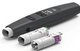
The PZ3 PiezoBrush is a compact hand-held plasma device that was developed for use in laboratories, advance development and assembly in short production runs. With a maximum power consumption of 18 W, Piezoelectric Direct Discharge (PDD®) technology is used to generate cold-active plasma at a temperature of less than 50 °C.
