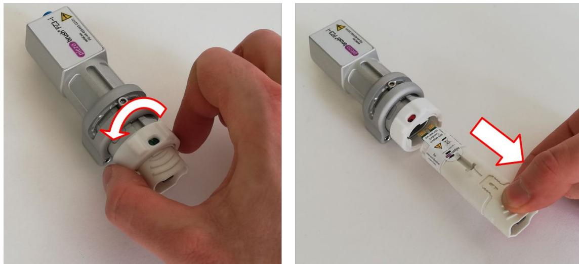
If the installation situation prevents the exchange module from being removed downwards when mounted, the module carrier including module can be removed without tools. To prevent damage to the module cable, we advise that you disconnect it before removing the module carrier.
