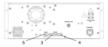
6. Connect the "USB-to-CAN" PC/CAN interface to the USB connection of your PC.
