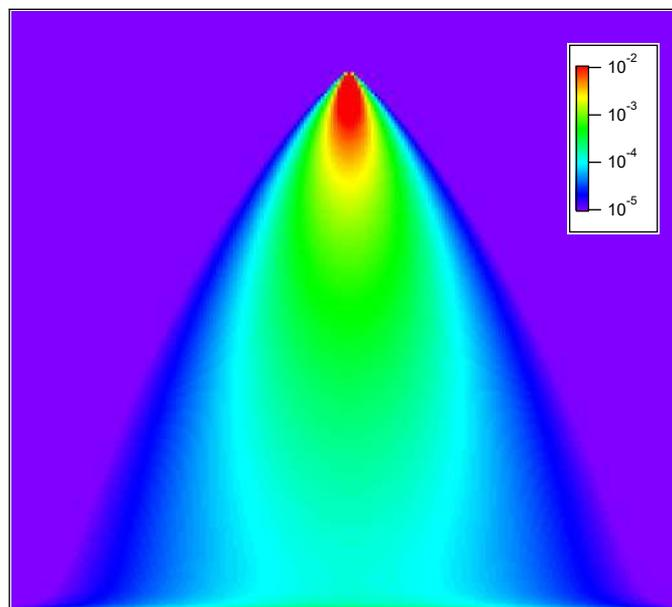
**Figure 7:** UV light exposure map (light emission of jet weighted with the spectral sensitivity according to ICNIRP) generated by a **plasma jet directed into an open environment** (bottom plate of the box assumed to be a diffuse lambert emitter). Field of view 2 m x 2 m.
