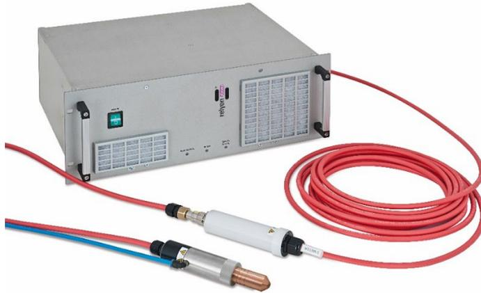
**Figure 1:** *The PlasmaBrush PB3 is a combination compact plasma jet generator nozzle and a unipolar pulsed high-voltage source used for industrial plasma process integration. Usually, it will be operated with air (CDA).*
