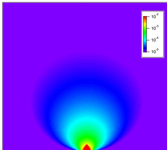
**Figure 8:** UV light exposure map generated by a **plasma jet directed onto a metallic substrate** (bottom plate of the box), acting as a diffuse lambert emitter without losses. Field of view 2 m x 2 m.
