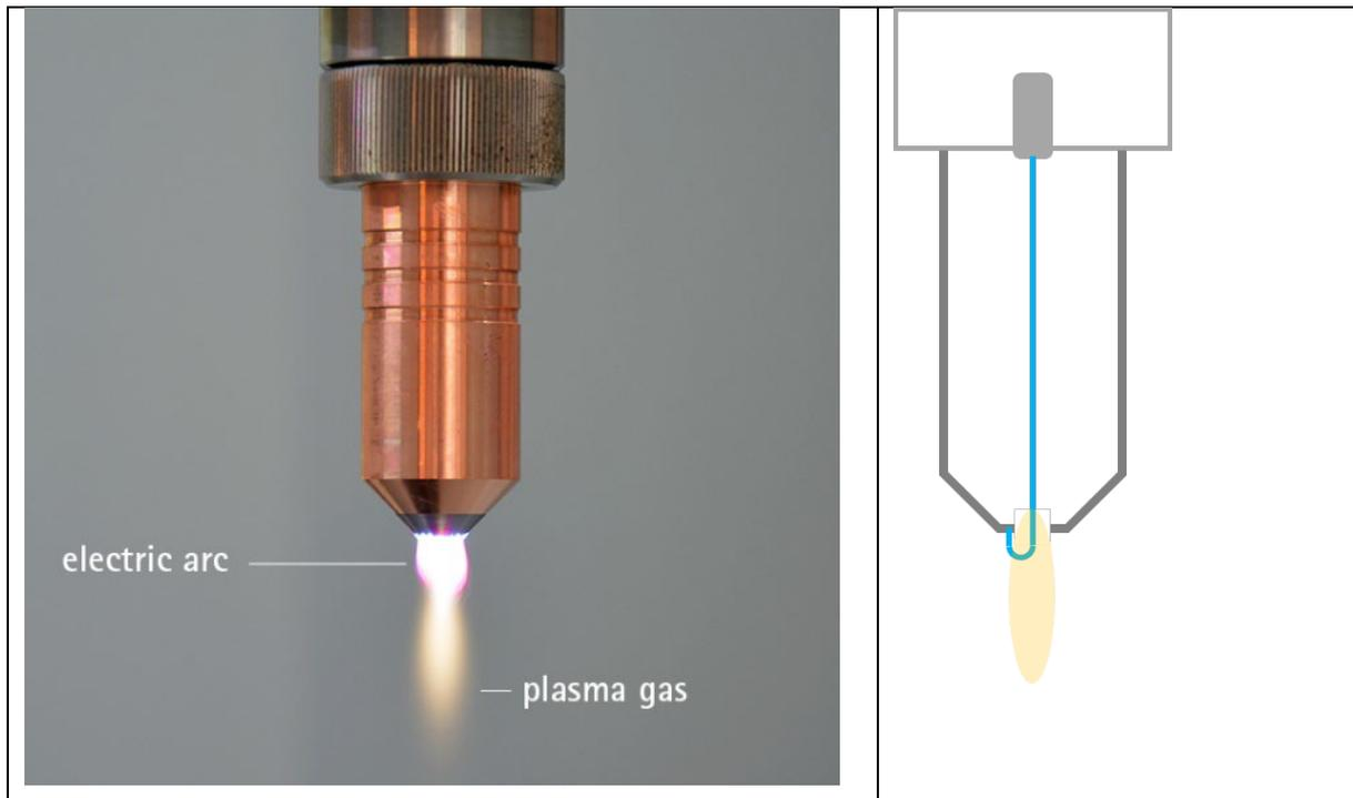
**Figure 2:** Photograph of the PlasmaBrush PB3 jet using the A451 nozzle operated at full power and an air flow of 50 slm. The right side depicts the simplified position of the filamentary arc stretching from the inner anode to the aperture of the nozzle-shaped copper cathode.
