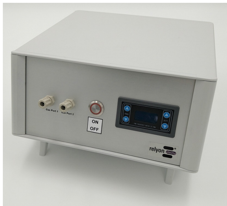
Figure 1: Front side with gas connectors, activation switch and power control unit
