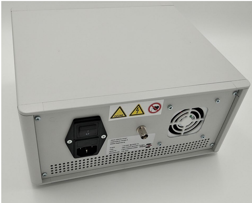
Figure 2: Back side with power socket, main switch, BNC signal out and cooling air outlet
