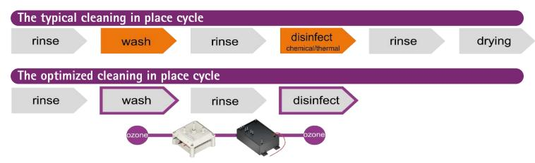
The typical cleaning in place cycle consists of six steps. By integrating ozone into the cleaning process, the process can be optimized by two steps. This eliminates the need for chemical agents or heat. The use of ozone thus makes it possible to save time, energy and resources for end users. These savings automatically result in cost savings.
