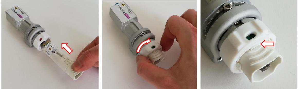
Grip the module carrier as shown and place it on the driver housing by sliding it onto the two locating pins from the front and then pressing it firmly home against the driver housing.
