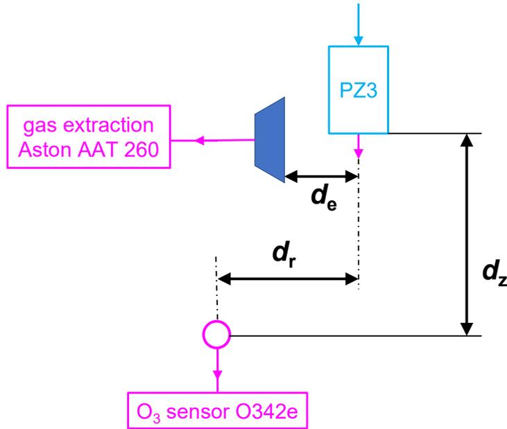
Figure 8: The geometrical configuration of instruments for measurement of the concentration of ozone generated by piezobrush<sup>®</sup> PZ3 for different positions in respect to the ozone sensor gas inlet and gas extraction conditions.
