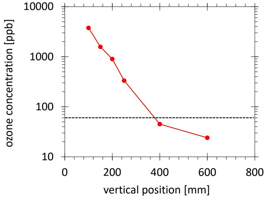
Figure 10: Mean concentration of ozone generated by piezobrush<sup>®</sup> PZ3 operated with full power (8 W) as a function of vertical distance between the sensor suction terminal and the piezobrush<sup>®</sup> PZ3, at a vertical distance of 250 mm.
