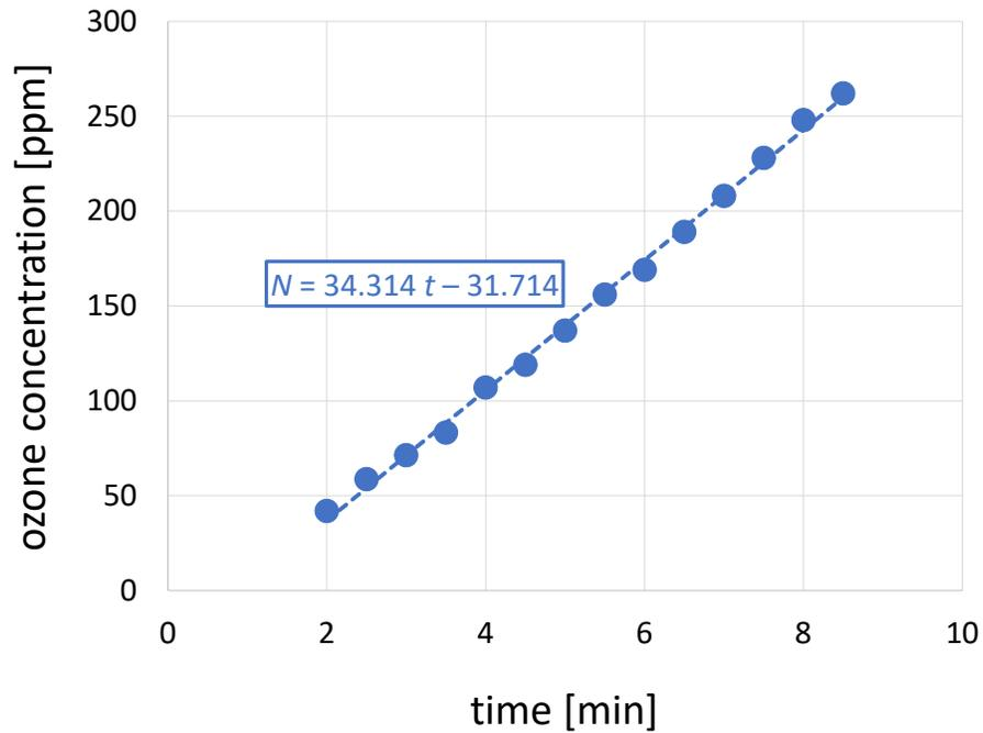
Figure 7: Ozone concentration as function of piezobrush<sup>®</sup> PZ2 operation time in 20 l bag.
