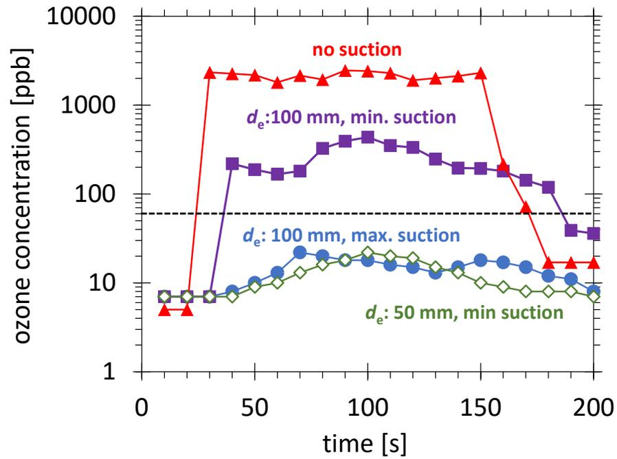
Figure 9: The time-dependent response of the ozone concentration on two minutes operation of piezobrush<sup>®</sup> PZ3 with full power (8 W), at constant vertical distance,  $d_z = 250$  mm between the piezobrush<sup>®</sup> PZ3 open nozzle and the ozone sensor gas inlet, for different distances  $d_e$  between the piezobrush<sup>®</sup> PZ3 open nozzle and the suction funnel, and different gas extraction power levels.
