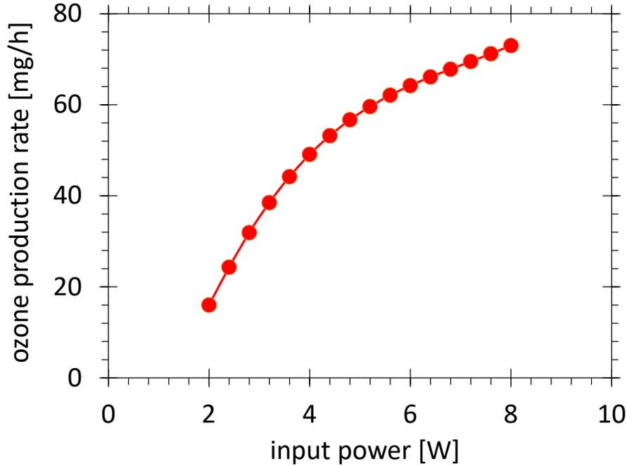
Figure 5: Ozone production vs. power of piezobrush<sup>®</sup> PZ3 operated with ambient air.
