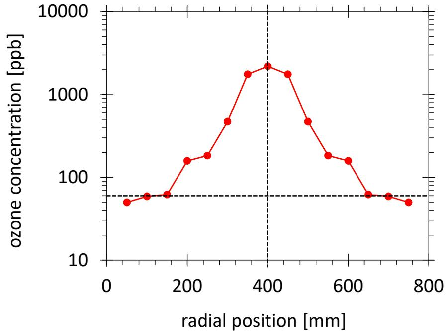
Figure 11: Mean concentration of ozone generated by piezobrush<sup>®</sup> PZ3 operated with full power (8 W) as a function of horizontal distance between the sensor suction terminal and the piezobrush<sup>®</sup> PZ3, at a vertical distance of 250 mm.
