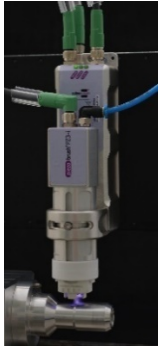
Picture 1: piezobrush ® PZ3-i device consisting of driver housing and module mount
