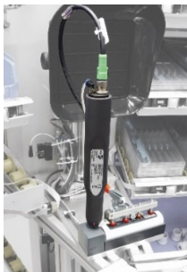
Picture 3: Use of the predecessor model piezobrush ® PZ2-i for bonding polypropylene (PP) Source: IKA ® -Werke GmbH & Co. KG
