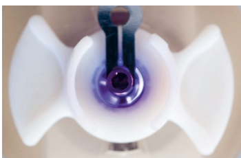
Picture 4: Plasma discharge on a dental implant in the implaPrep concept
