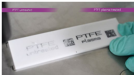
Image 2: Adhesion test of inkjet printing on untreated and plasma-treated PTFE
