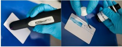
Image 3: Examination of surface energy using test inks before and after plasma treatment
