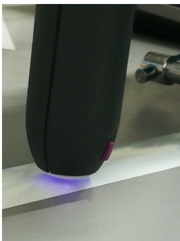
Figure 2: piezobrush PZ2 during activation of the PSA coated strip of foil.
