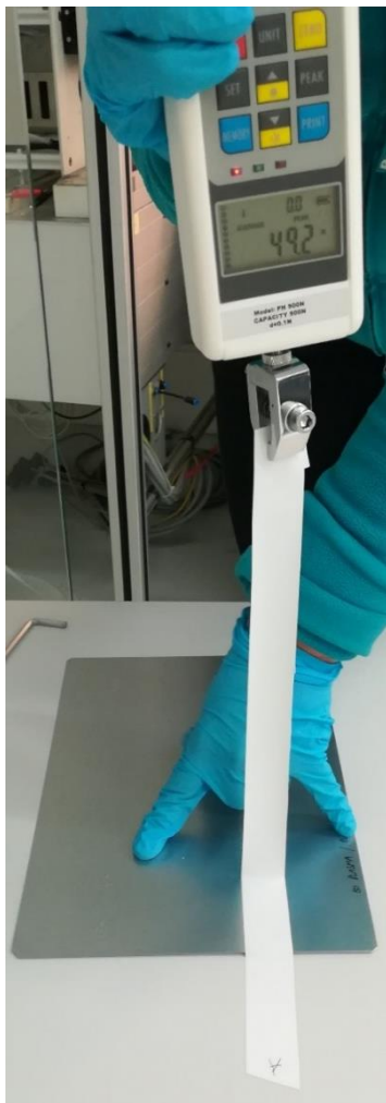
Figure 3: Conduction of the peeling strength test.
