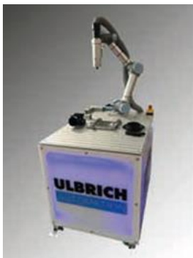
Image 4: Mobile 6-axis collaborative robot system for dosing and surface treatment with plasma
