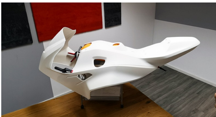
Image 3: Motorcycle fairing printed in twelve individual parts, treated with plasma and glued together
