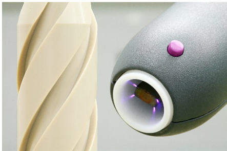
Image 2: PEEK implant during treatment with the piezobrush PZ2
