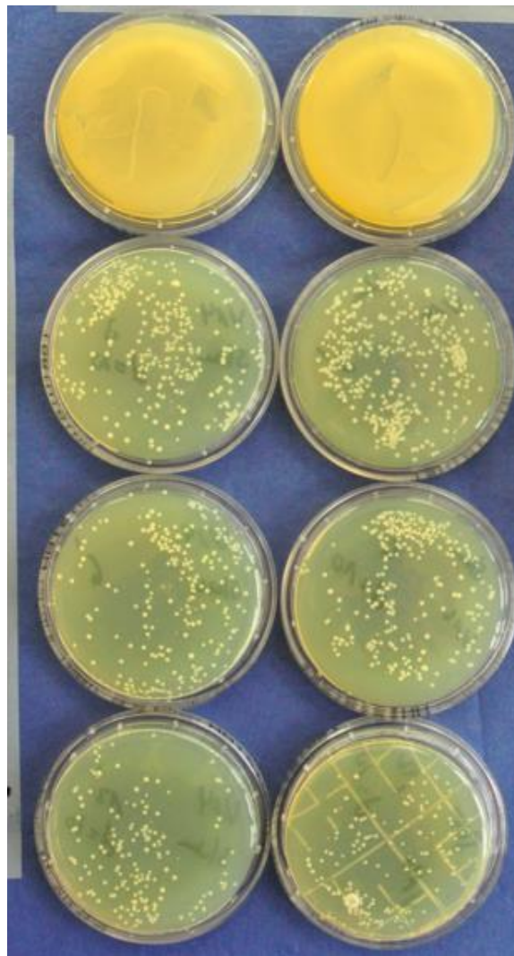
Fig. 5. Two similar time series of dry air plasma treated S.A. culture at 50mm distance with 6L/min airflow and exposures of 1min, 2min, 6min against the reference first row.
