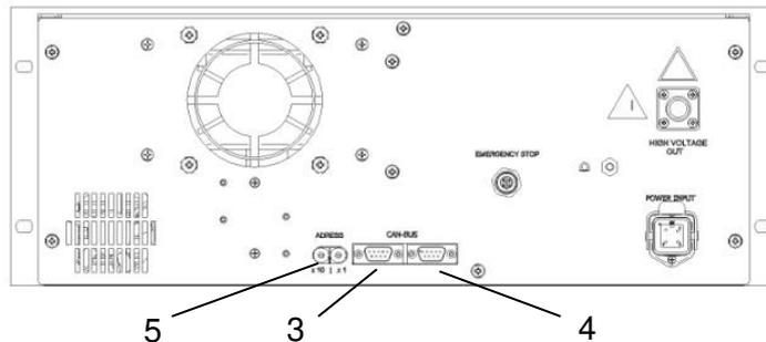
6. Establish the emergency stop circuit for the PS2000 and all other connections of the additional machines as described in the corresponding operating instructions.
