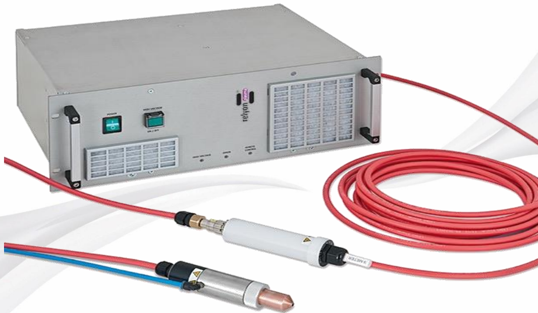
Picture 1: Plasma system consisting of a 19-inch power unit for the high voltage supply (PS2000), a robust and flexible connecting cable, and the compact plasma generator PB3 with nozzle insert (A450). The system can be operated using air, nitrogen and reductive forming gas (H 2 /N 2 ).
