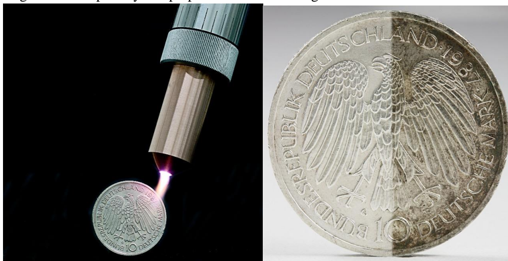
Picture 4: Reduction of a silver special edition coin. Left: size comparison of the coin and the plasma jet at the nozzle exit. Right: effect of the reductive plasma treatment (5% H 2 /95% N 2 ) on the coin, which was half masked prior to treatment. The effect is achieved after only about 1 second of treatment (cf. Schmitt-Ott, 2009).
