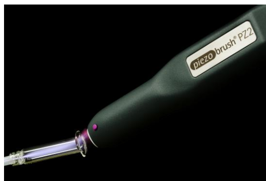
Fig. 3. PZ2 igniting an intense glow discharge in a glass cavity purged with Ar/O 2 .
