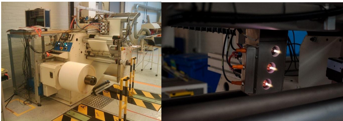
Picture 4: Treatment of aluminum foil in a roll to roll procedure
