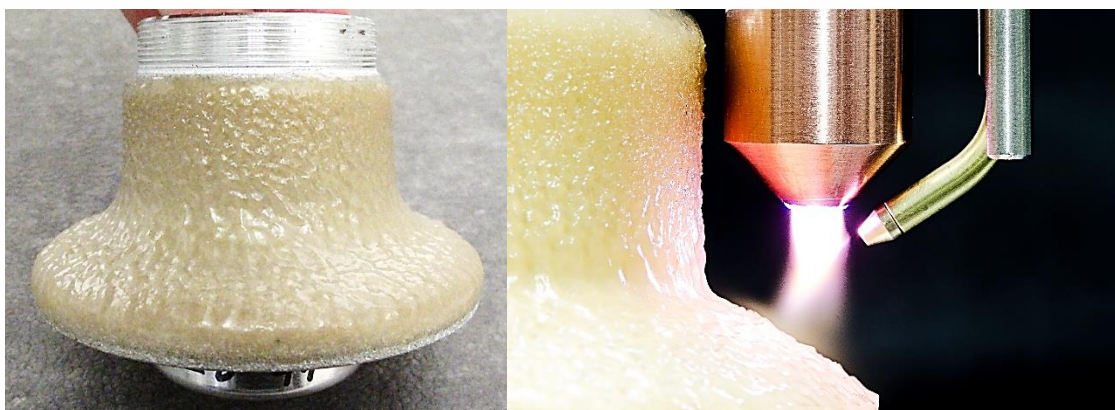
Picture 5: Completed hot melt coating (left) and Plasmabrush ® with external injection (right).
