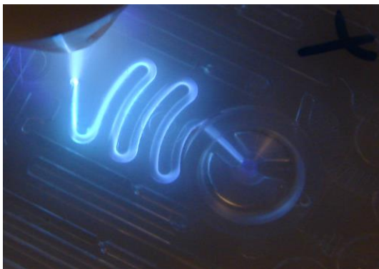
Picture 3: PZ2 handheld device in laboratory use for the pretreatment of dental materials (inorganically filled synthetic resins, PEEK, titan).
