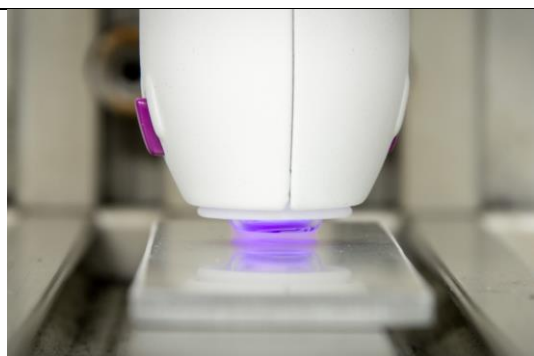
Surface treatment of a glass test item using piezo brush ® PZ2. Treatment duration is ca. 5s/cm 2 .
