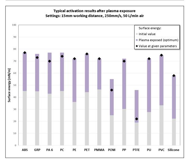
**A450** typical activation results for the given parameter set of speed and working distance operating with air. Higher surface energies through process parameter ajustment can be achieved.
