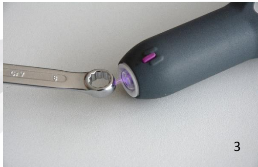
Picture 2: Nozzle caps for various applications. (1,2) Needle nozzle for inside treatment of pocket holes, cavities and for using special gases. (3, 4) Nozzle insert for extensive treatment of sensitive or conductive surfaces.
